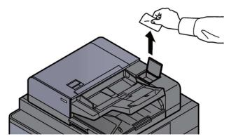
Clean the slit glass surface and the reading guide.
