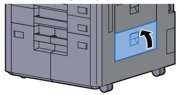
11 If the optional side feeder is installed, return the side feeder to the original position.
