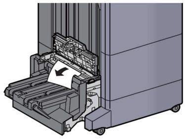
1 1 Open the folding unit conveyor guide.
