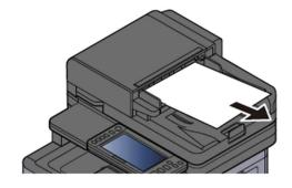
Open the Document Processor cover and remove the jammed paper.
