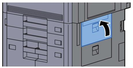
If the optional side feeder is installed, return the side feeder to the original position.
