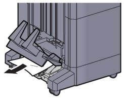
12 Press the release lever to pull the folding unit out.
