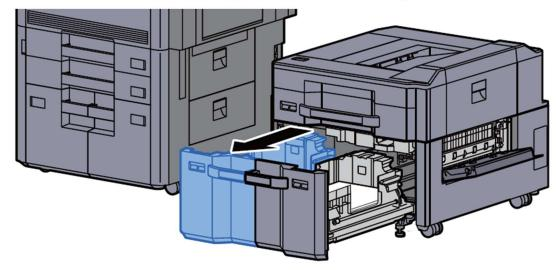
7 Pull out side feeder paper feed unit (B1).
