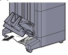
12 Press the release lever to pull the folding unit out.
